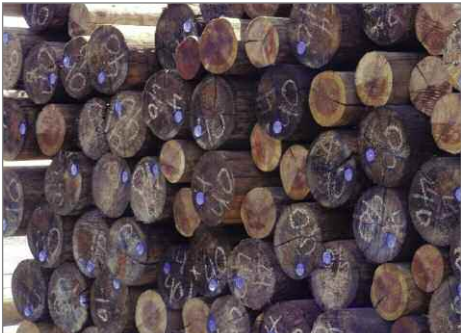
A bin of dry and framed ready-to-treat poles.
