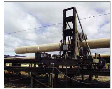
One of the out feed carts at the pole peeler.
