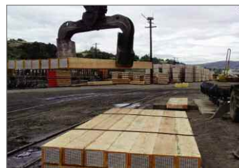
Amerities stacks and treats over 700,000 hardwood and Douglas fir cross ties, switch ties, and bridge timbers annually for Union Pacific Railroad.
