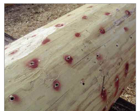
Radial pattern drilled poles.
