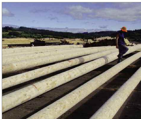
Doug fir poles are ready for drilling and framing.
