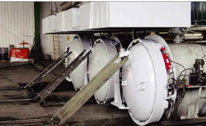
Rainier is one of three plants that can treat with ACZA in three retorts at a current capacity of 300,000+ Douglas fir ties annually. This plant is also responsible for producing several million feet of dimension lumber/timbers for retail.
