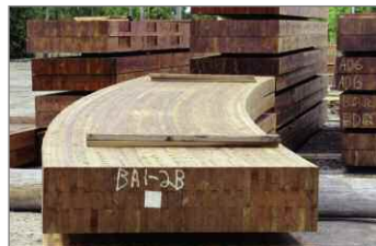
JH Baxter's specialty is custom work and large materials such as these penta-treated glu-laminated square utility transmission poles and bridge arches.
