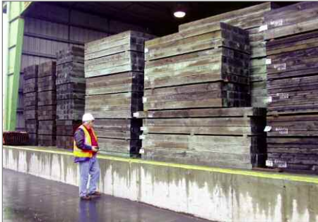
ACZA-treated cross-ties and switch-ties along with some dimensional lumber. The material stays under cover until dry, before moving to storage.
