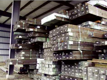
ACZA-treated timbers for Marine Splash use with much higher retentions than the cross-ties.
