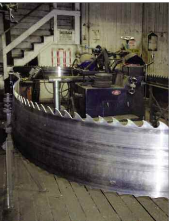
The nine-foot band saw blades are sharpened regularly for the moving head rig carriage.
