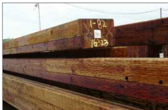
JH Baxter's specialty is custom work and large materials such as these penta-treated glu-laminated square utility transmission poles and bridge arches.
