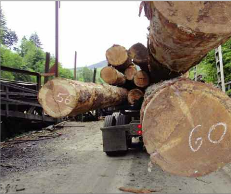
Incoming logs, a 56' and 60', are unloaded into the log holding pond before peeling.
