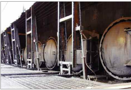
Five 7' x 132' creosote pressure treating retorts at this Amerities facility are used for both UPRR (90%+) and some commercial business.
