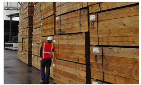
Green No. 1 Douglas fir cross-ties and switch-ties at one of Conrad's three treating facilities in Washington and Oregon. Rainier inventories 20,000+ ties.
