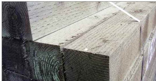
...then we have a look at some ACZA-treated timbers. This plant treats with oilborne and waterborne systems.
