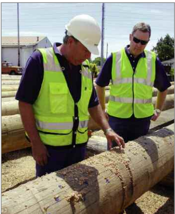
Reniff and Tolko's Jamie MacMillan inspecting poles have been drilled to increase preservative penetration.
