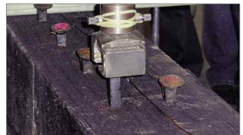
Spike pull test from a tie exposed outdoors for two years at the OSU field test site near Corvallis.
