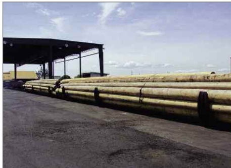
A charge of transmission poles staged for treating.
