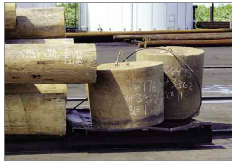
Two 2-ton Penta blocks loaded onto trams for mixing in the retorts.
