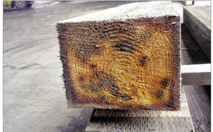
No. 1. Grade WCLIB Douglas fir treated to AWPA standards. This particular piece was taken from a random unit of ties for the benefit of the group and cut before arrival.
